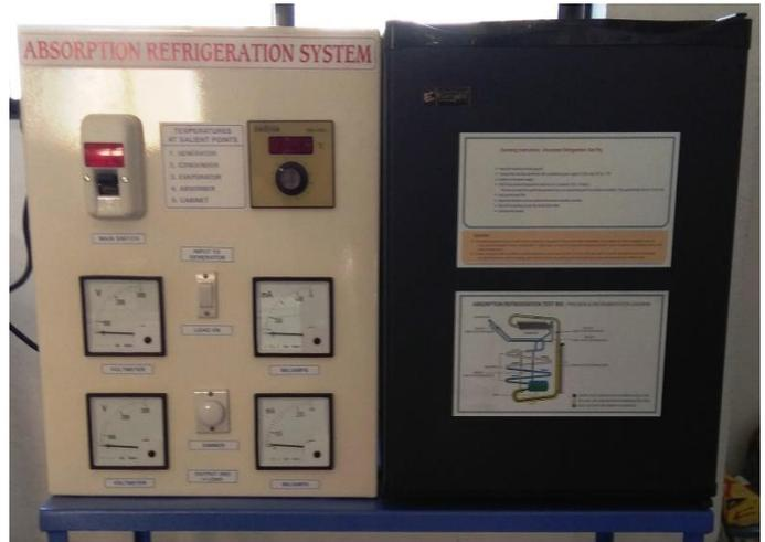
Refrigerating plants make use of the fact that a refrigerant evaporates at low pressure. In absorption refrigeration systems, the absorption of ammonia in the water produces this low pressure. The absorption process is driven by thermal energy, which can come for example from industrial waste heat or solar collectors to operate these systems.
