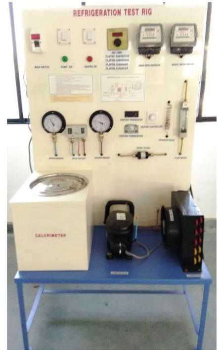
The rig incorporates a hermetically sealed compressor provided with an air cooled condenser and an evaporator with water as a medium and heater. Evaporator temperature is kept constant by adjusting the heater and heater input is taken as refrigerating effect. With various measurements, Actual COP, Theoretical COP, Carnot COP and heat transfer coefficient in evaporator can be calculated.
