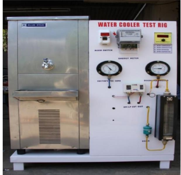
The water cooler consists of an insulated stainless steel tank around which evaporator tubes are wound and soldered. The tubes are made of refrigerated grade annealed copper tubes. This is a direct expansion type evaporator. The heat absorbed by the refrigerant is passed through water which is continuously flowing.
